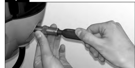
To start cleaning process, while holding Quick Clear Adapter in place, unscrew the Quick Clear cartridge 1/4 Turn Only.
